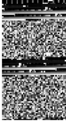
Figure 1: Byteplot visualization from a Windows thumbs.db file depicting significant structural differences between header information and compressed image data (seen as white noise).
